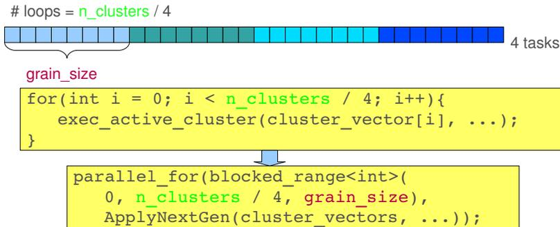
Figure 5: Parallelization with TBB
