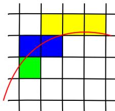
Figure 1: The triggering of pads from a track.
