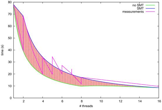
Figure 12: Execution time of tbb benchmark on Xeon X5570 using #threads
