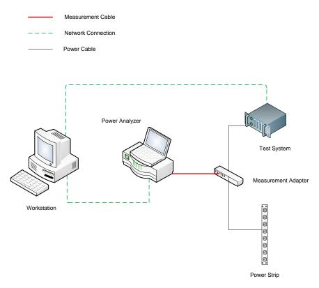
Figure 2: Power test setup
