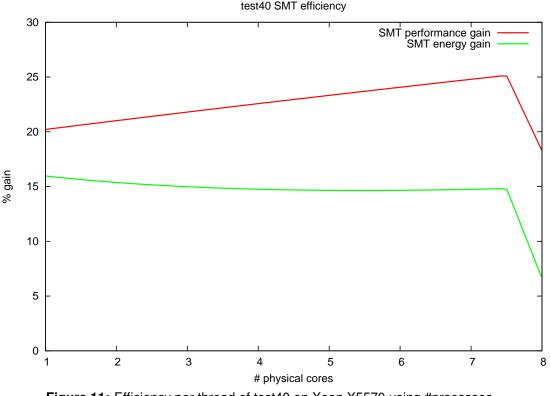
Figure 11: Efficiency per thread of test40 on Xeon X5570 using #processes
