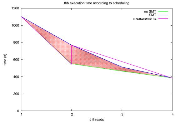
Figure 16: Execution time of tbb benchmark on Irwindale 3.6 GHz using #threads
