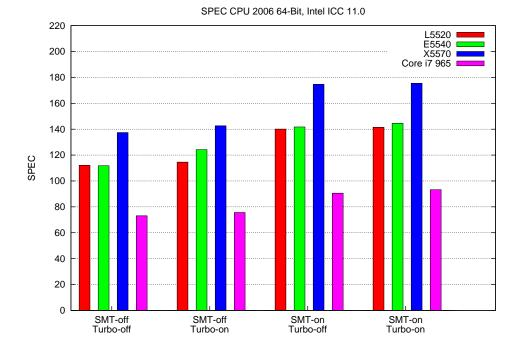
Figure 7: SPEC CPU2006 results of Xeon 5500 and Core i7 965 for Intel ICC 11.0, 64 Bit
