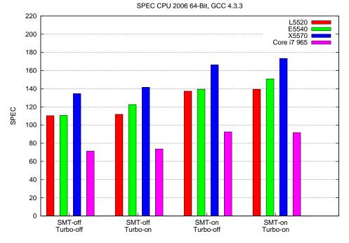
Figure 5: SPEC CPU2006 results of Xeon 5500 and Core i7 965 for GCC 4.3.3, 64 Bit
