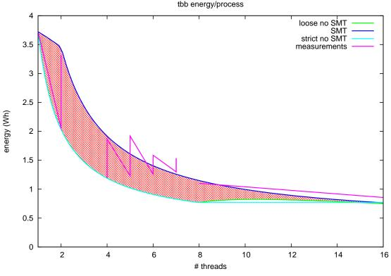
Figure 13: Energy per thread of the tbb benchmark on Xeon X5570 using #threads
