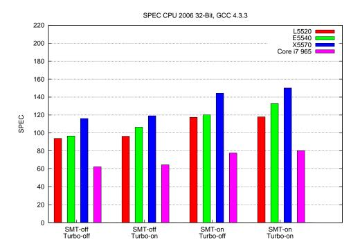
Figure 4: SPEC CPU2006 results of Xeon 5500 and Core i7 965 for GCC 4.3.3, 32 Bit
