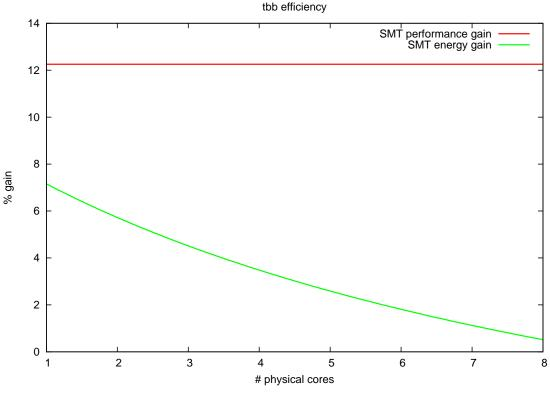
Figure 14: Efficiency per thread of tbb benchmark on Xeon X5570 using #threads
