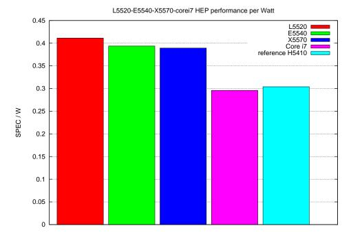
Figure 8: Efficiency of Xeon L5520, E5540, X5570, Core i7 965 (SMT-off, Turbo-on) and Harpertown H5410 (GCC 4.1.2, 32 Bit)
