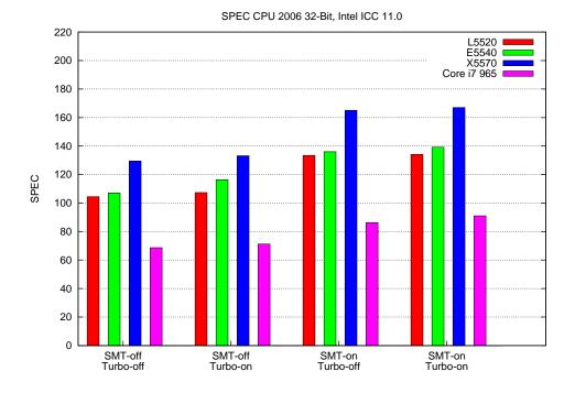
Figure 6: SPEC CPU2006 results of Xeon 5500 and Core i7 965 for Intel ICC 11.0, 32 Bit
