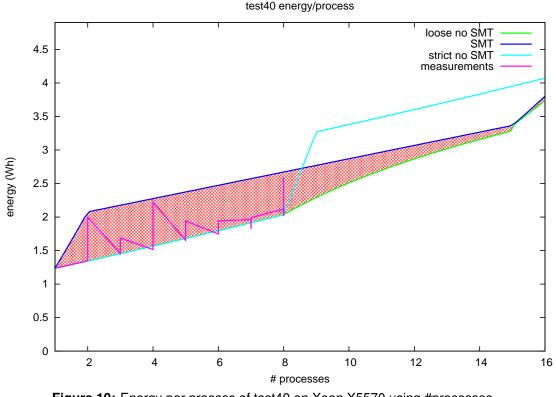
Figure 10: Energy per process of test40 on Xeon X5570 using #processes
