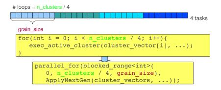
Figure 5: Parallelization with TBB
