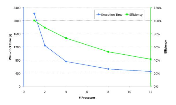
Figure 8: Time spent for the calculation of the fit application (blue line) and efficiency (green line).
