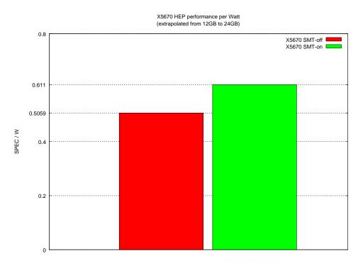
Figure 4: Efficiency of the Westmere platform with a single PSU
