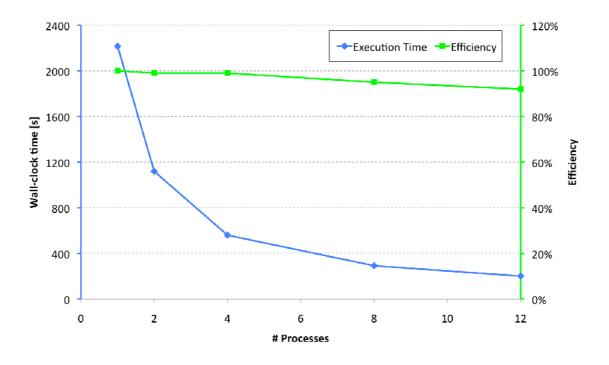
Figure 9: Time spent for the calculation of the fit application (blue line) and efficiency (green line). For this plot we subtract the time spent for the extended term calculation.
