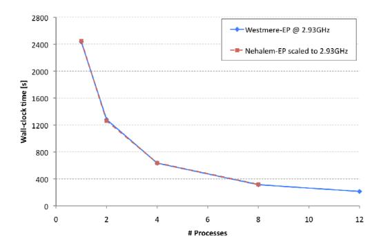
Figure 10: Execution time (only computational part of the application excluding the extended term calculation) for the Westmere-EP (solid blue line) and Nehalem-EP (dashed red line). Both results are scaled to 2.93GHz.
