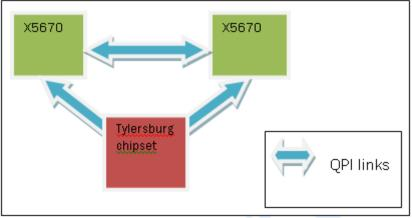
Figure 1: QPI connections
