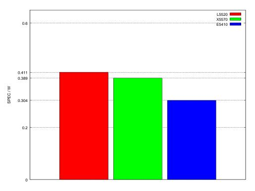
Figure 5: Efficiency of the Nehalem microarchitecture SMT-off
