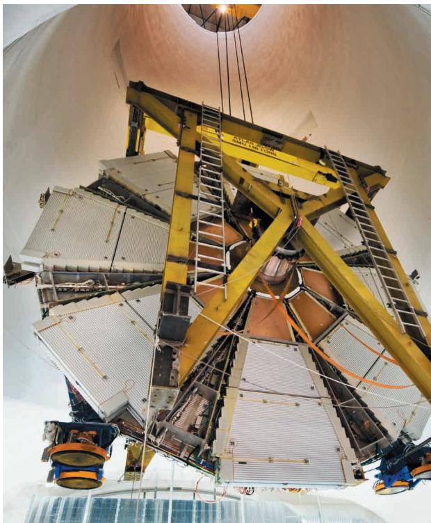
Small wheels of the ATLAS muon spectrometer
