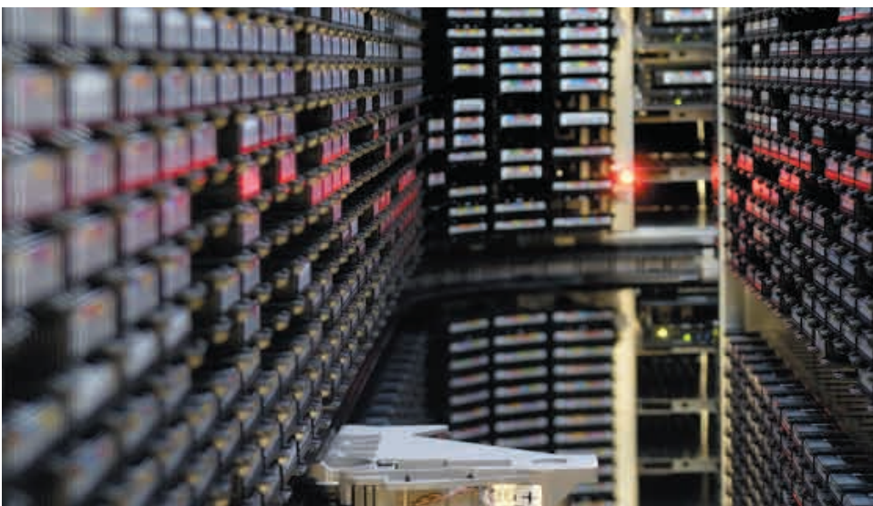
Database systems for the LHC Computing Grid must keep track of files stored both on disk arrays (opposite page) and in tape storage systems (this page) at CERN and in the 11 major Tier-1 centres.
