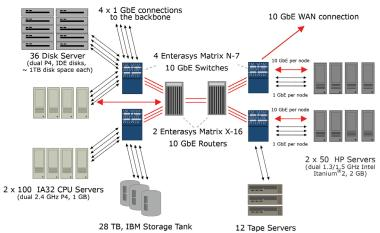
IBM sponsored 28TB of high-end SCSI storage together with the IBM TotalStorage SAN File System storage subsystem. In its largest configuration the subsystem was equipped with 15 storage controllers.
