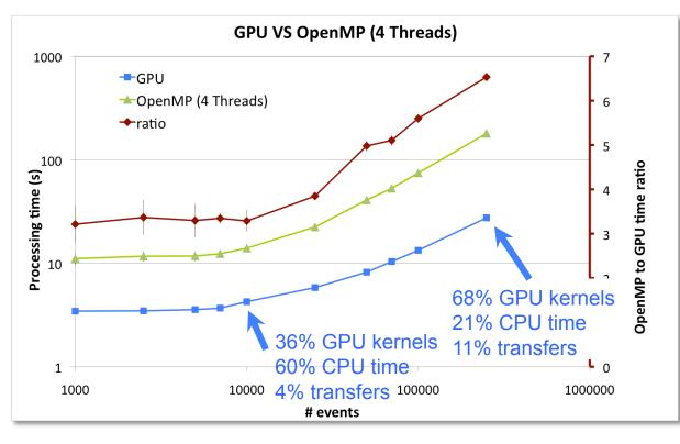
Speed-up increases with the dimension of the sample, taking benefit from the data streaming on GPU and the integral calculation only on the CPU
