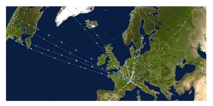
up to 1 Gigabyte/s. This data rate corresponds to transferring a DVD worth of scientific data from CERN every five seconds. The data was transferred around the globe using 10Gbit/s private optical networks linking CERN to the 11 Tier-1 sites. When it is fully operational, the LHC will produce about 15 million Gigabytes of data annually.
